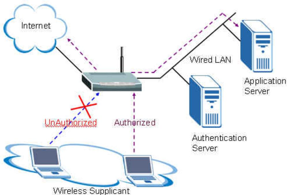
The IEEE 802.1x authentication is a client-server architecture delivered with the EAPOL (Extensible Authentication Protocol over LAN). The authentication server authenticates each client connected to an Access Point (for Wireless LAN) or switch port (for Ethernet) before accessing any services offered by the Wireless AP. The 802.1x contains three major components:
