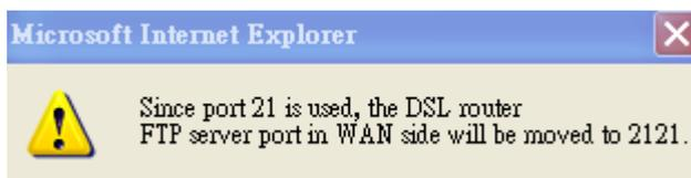
This phenomenon is normal, because the CPE itself can be accessed by the FTP, which the port is also 21. Since we are creating a new rule using port 21, the default port number of the CPE's FTP server port will automatically be moved to 2121.
